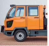
Modern, ergonomically designed space-frame cab with unimpeded view of the working equipment and surrounding area as well as a crew cab for transporting up to five persons
