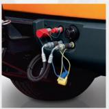
Attachments are driven by the vehicle's powerful hydraulics – and easily connected to non-drip, flat-sealed, quick-connecting couplings
