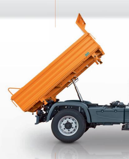
Balanced handling and secure roadholding whether in a loaded or unloaded state due to the independent suspension with helical springs at the front and progressive leaf springs with telescopic shock absorbers at the rear
