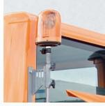
Telescopic flashing beacon on a stand (either one or two)
