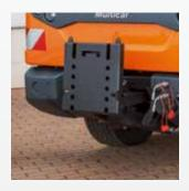
Three different attachment points, front-mount quickchange system with lifting and lowering functions for easy loading of various front-mount devices
