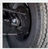
Balanced driving- and safe road holding characteristics whether fully loaded or empty - due to an independent suspension with coil springs at the front and progressive flat springs with telescopic shock absorbers at the rear
