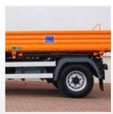
Tipper superstructure ball-mounted on cross beams, ball-change system for quick mounting/ dismounting of superstructures components
